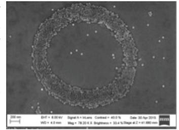
2.5 micrometer diameter toroidal magnet assembled from 30 nm diameter magnetic nanoparticles using perpendicular recording medium (Crawford group)
